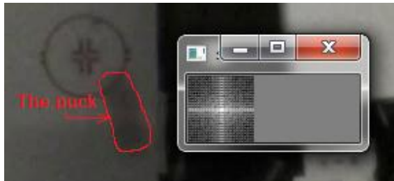
Figure 3. The Fourier transform of FR and the resulting DC values on horizontal and vertical axes
