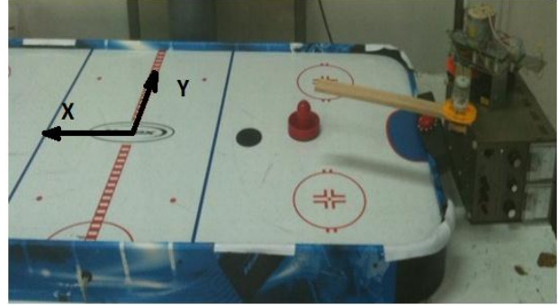
Figure 1. The air hockey table with its goal, paddle, puck. The paddle has been colored in red and the puck in black (on front of paddle). A 2DOF robot is supposed to use the velocity estimation by an off-the-shelf camera to predict the position of the puck and block the goal.
